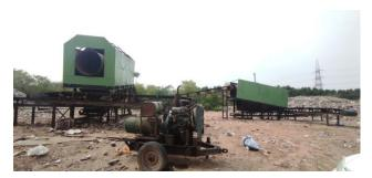
FIGURE 3.2: Waste segregation or sorting machine
